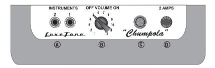
(A) INSTRUMENT CHANNEL INPUTS — Plug-in connection for instruments.
